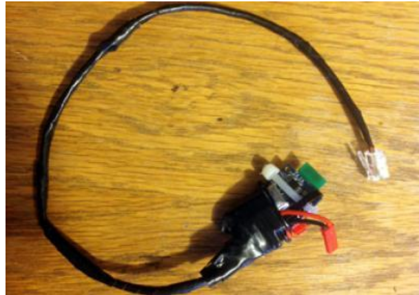
Cui's makeshift tool to inject malware into Cisco phones
