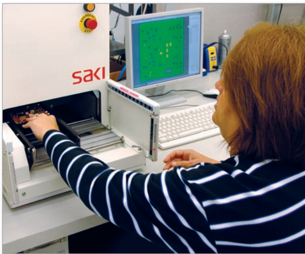
A high resolution automated optical inspection system is one of several tests used to analyze circuit boards for quality and consistency.
