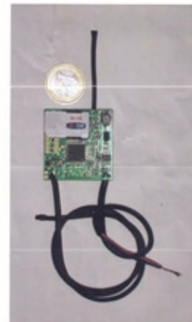
GSM Based Audio Eavesdropping Device discovered on a major Corporate Jet Aircraft UK 2008
