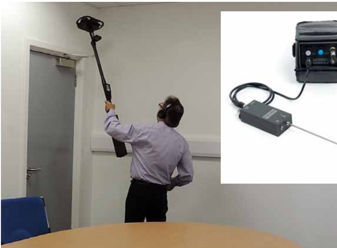
The Shearwater Bloodhound can be used to sniff out hidden listening devices
