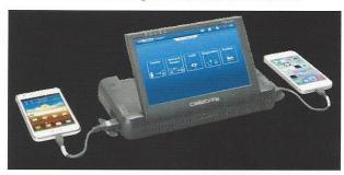
The RAPTOR RXi counter-surveillance receiver stands out from the crowd due to its wide scanning frequency range of 10kHz to 26GHz, 20MHz real-time bandwidth, wealth of functionalities and large (15") colour touch screen display.
