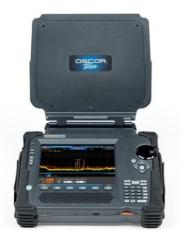
detect transmitting electronic surveillance devices and ensure that spectrum activity is captured.
