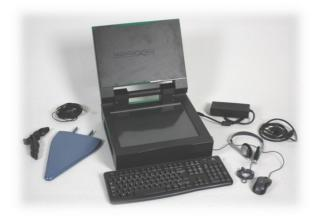
Featuring a fast Core 2 Duo processor, its multiple software tools and demodulators detect frequencyhopping, burst mode and spread spectrum devices as well as analogue audio and video signals. The 'Waterfall' display mode gives an intuitive display of signals over time. The RXi is fully portable, operating either from an internal rechargeable battery or an external supply. Its integrated antenna system provides wideband performance from 10 kHz to 26GHz.
